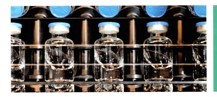
From the infeed system, the product is conveyed through the inspection cabin on a continuously or intermittently moving transport system, consisting of a dual chain system fitted with rollers. Each roller has telescoping shafts which allow easy removal and repositioning on different pin positions to accommodate a wide range of containers of various sizes. In addition to different lighting systems, top and
